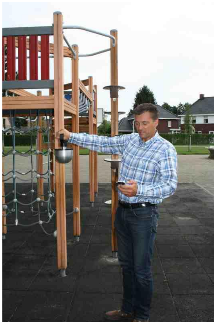
Wireless Bluetooth Impact Drop testing to AS4422 being performed by Playtest
